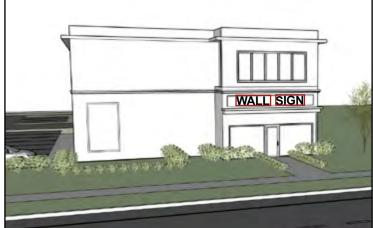
155.065 (3). Example of the measured area of this wall sign is highlighted by a red box. The box is drawn around the individual words that make up the sign. Addtional elements, such as symbols, logos, or any related components that make up the total sign would be measured similarly with geometric boxes as appropriate.
